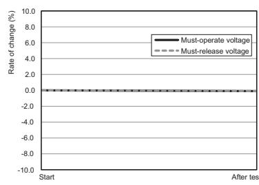
Characteristics were measured after applying a shock of 490 m/s<sup>2</sup> to the test piece 3 times each in 6 directions along 3 axes. The percentage rate of change is the average value for all of the samples.
